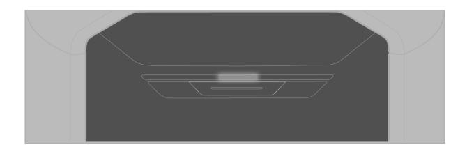
When the status LED displays an inwards running pattern, it means the extra battery is shutting down.
