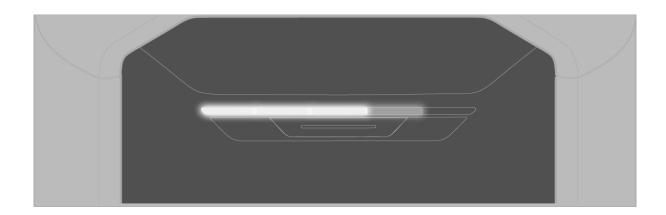
When the entire status LED is blinking, it indicates that an error has occurred.
