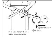
Next, hold the bent portion of the leg and insert one side of the joint pin head into the keyhole-shaped hole. Apply force to the 1 leg in the direction of the arrow and insert the head of the 2 joint pin into the keyhole-shaped hole
