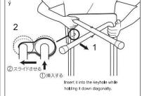
Confirm that the three joint pins are securely inserted, and insert the head of the joint pin into the keyhole-shaped hole in the same way as in ÿ. At this time, firmly fix the legs and top plate by hand so that the joint pins inserted in
